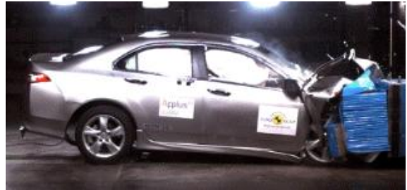
Offset crash test at 64km/hr
